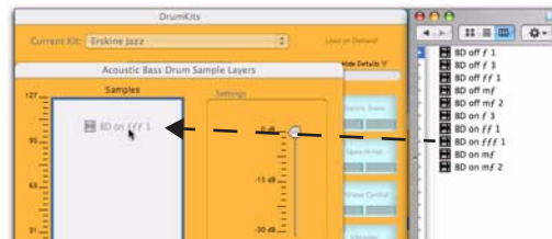
Dragging and dropping an audio file from the Desktop to a sample layer in DrumCore
